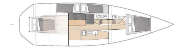
This arrangement shows the two bathrooms forward and once again is interchangeable with the aft cabin and open cockpit versions
