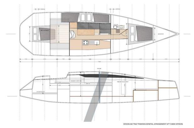
TR42 Trimaran Layout with single forward bathroom. The arrangement in the main saloon is interchangeable with the aft cabin and open cockpit versions.
